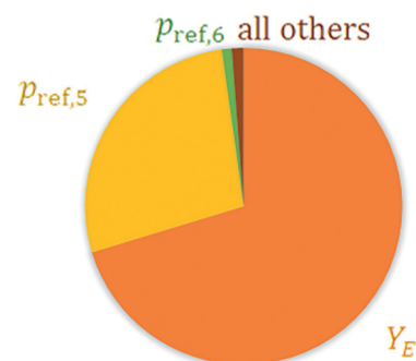
Fig. 8 Relative importance of the stochastic model parameters with respect to the reliability of the tunnel lining.
